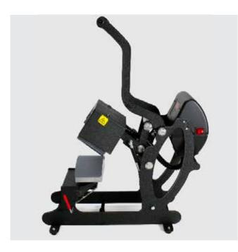
Locate the lift handle and position the heat platen in the UP position.
