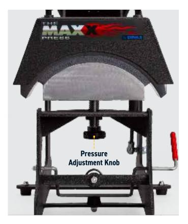
The Pressure Adjustment Knob is located directly under the lower platen.
