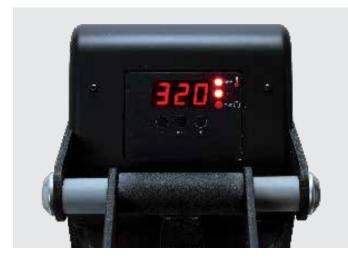
Press the Mode Select button in the center of the Control Panel.
