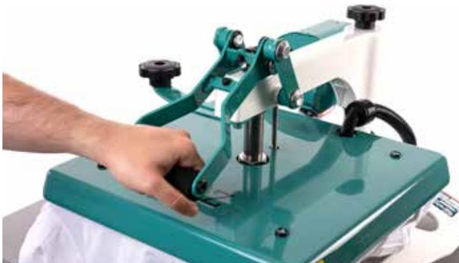
Lower the print handle fully until the upper platen locks into the press position. After the recommended pre-press time has elapsed, lift the print handle.
