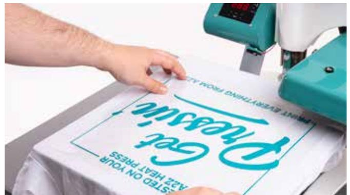
Swing away the upper platen and align the transfer on the garment.
