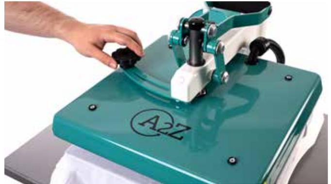
Some transfer products recommend a “pre-press” to heat and flatten the garment before printing. Using the swing handle, position the upper platen over the garment.
