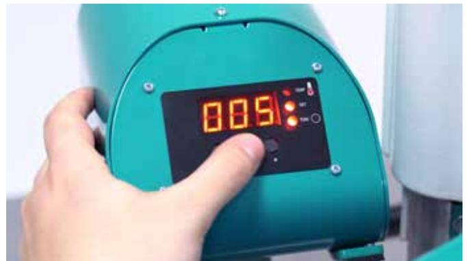
Press MODE twice to set the TIME. While SET and TIME are illuminated, press (+) and (-) buttons to adjust the TIME.
