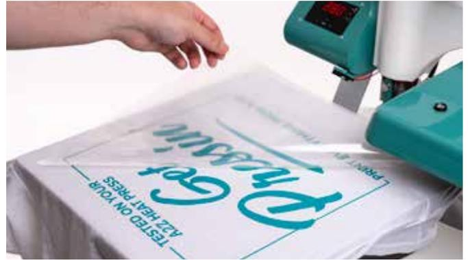
Using the swing handle, move the upper platen to access the garment. Depending on the transfer, peel the carrier hot or cold.
