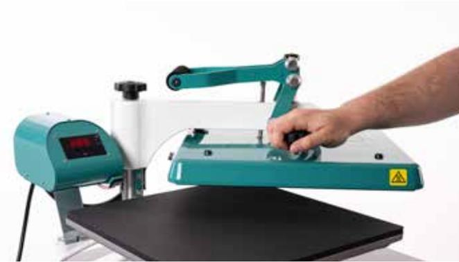
Using the swing handle, move the upper platen to access the lower platen. While heating, the print handle should remain raised to extend the life of the silicone pad.
