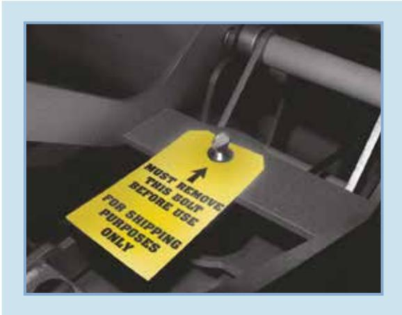
Locate the packaging bolt positioned on the top-centre of the press. Packaging bolt must be removed prior to turning the press on or operating the press.
